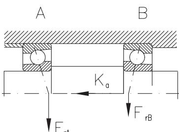
For bearings in DB and DF arrangements, the following equations are available:
