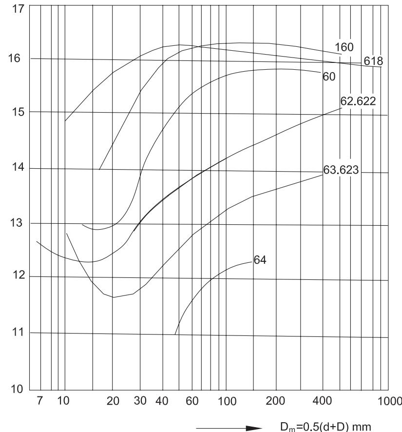
Calculation factors e, X and Z for deep groove ball bearings, single mounted or matched in tandem
