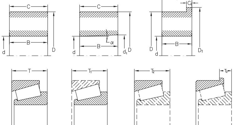
**Radial bearings (excepting tapered roller bearings)**
