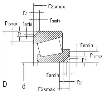
**Mounting chamfer dimension limits for tapered roller bearings**
