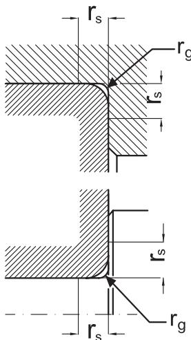
**Abutment dimension for Double row Cylindrical Roller Bearings**
