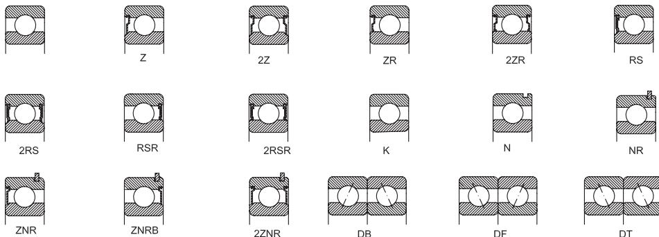
Besides deep groove ball bearings of basic design, bearings with UG design, with grooves on the outer ring and WL design, with grooves on both rings are also used for the purpose of mounting seals or shields on the bearings 2ZR, 2RSR or 2RS type, as shown in the bellow figure.
